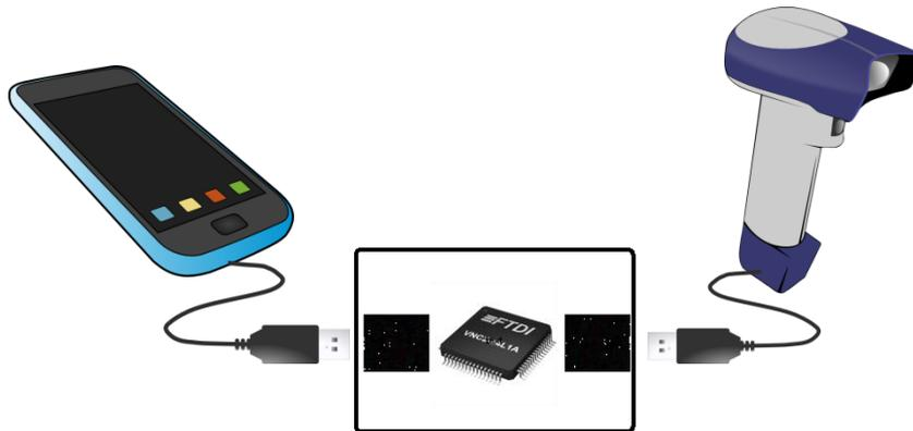
**Figure 2.3 USB Peripheral through Android Open Accessory**
