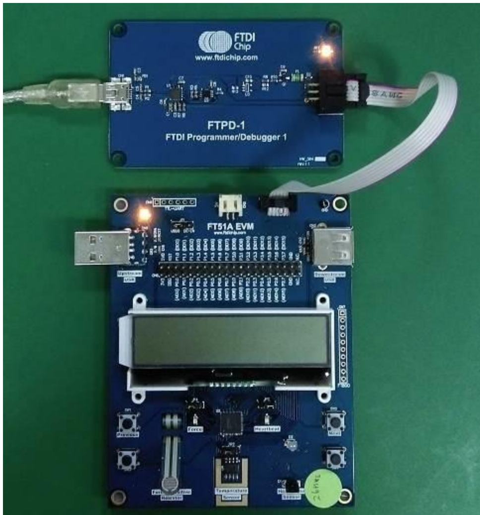
Figure 4 - FTPD-1 connection to UMFT51A-EVM
