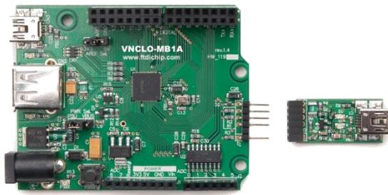
**Figure 3 : Vinco Development Module with VNC2 Debug Module**
