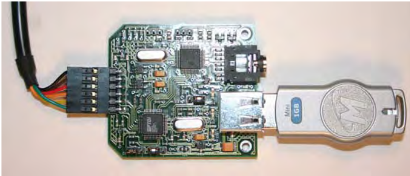
Figure 5.3: USB-to-Serial cable connected to VMusic board
