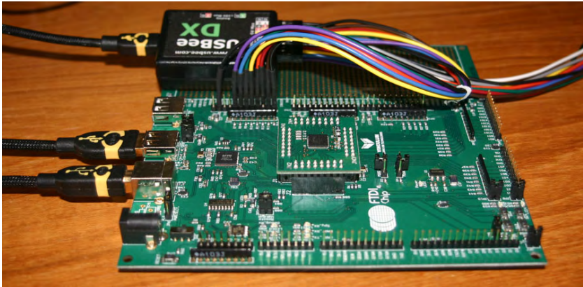
Figure 8.4: Connecting the USBee LA to the V2EvalBoard
