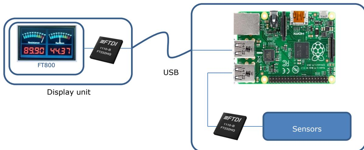
**Figure 2.2 Measurement system**
