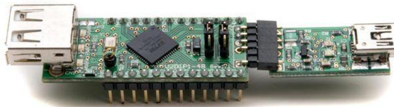
**Figure 3.1 V2DIP1 connected to the VNC2 Debugger/Programmer Module**
