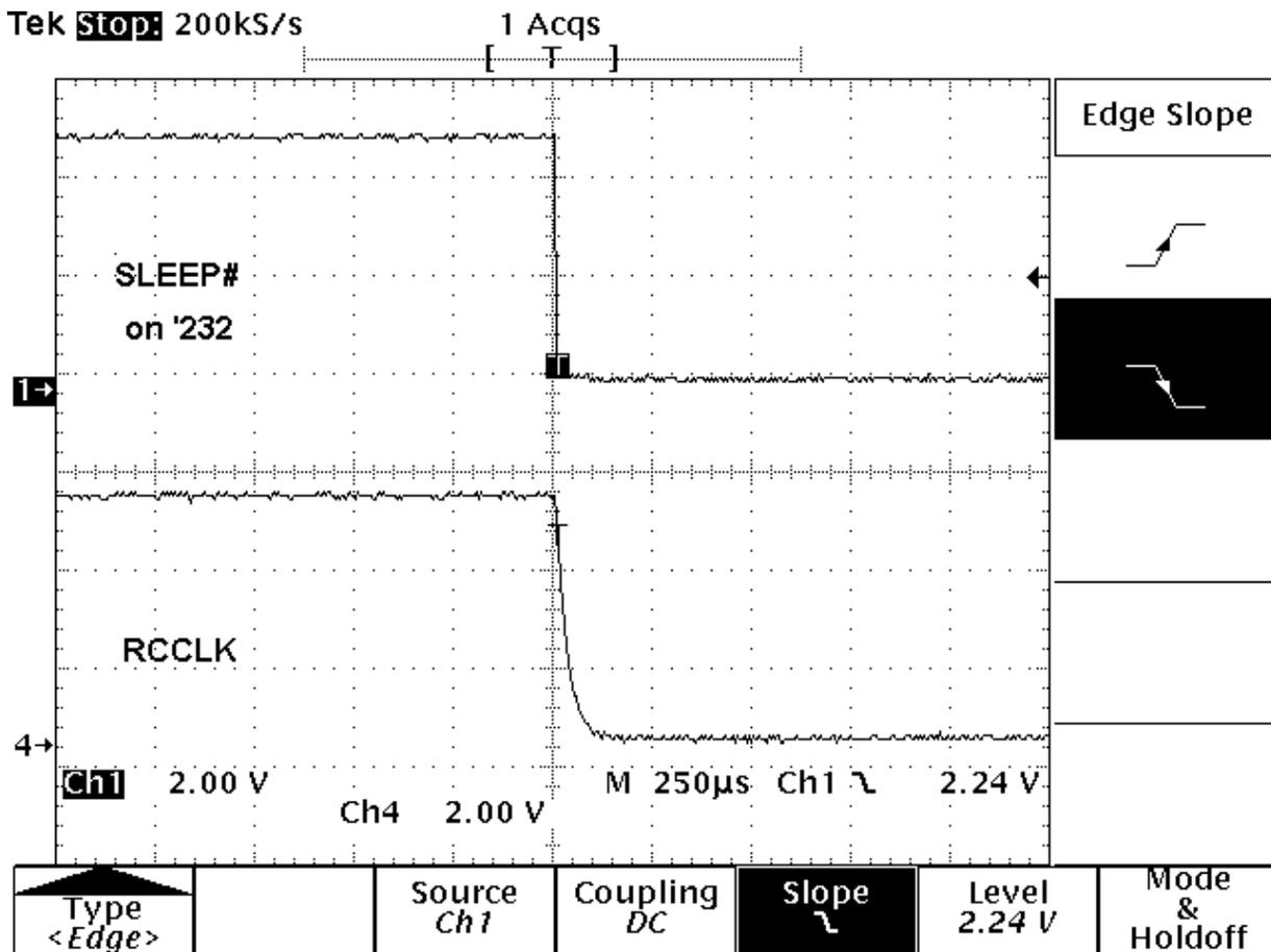
When the device wakes up to an external event such as USB resume or reset, it will release the RCCLK pin and use it to wait until the oscillator is stable.
