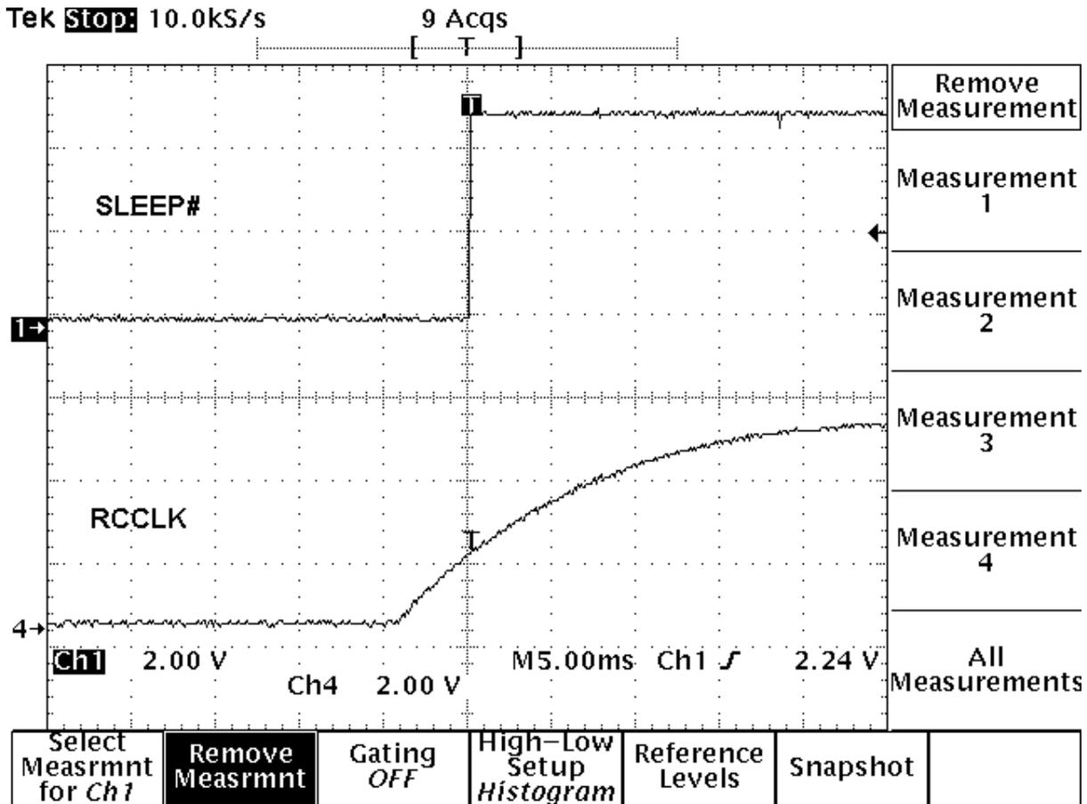
These next two diagrams show the relationship between RCCLK and the crystal oscillator. The frequency of the clock signal appears low because the digital oscilloscope is sampling too low to accurately reproduce it. It is a reasonable assumption that if the wave looks good at this sample rate then it will be good at its real frequency due to the oscilloscopes under sampling (i.e. if it appears to be oscillating, then it is).
