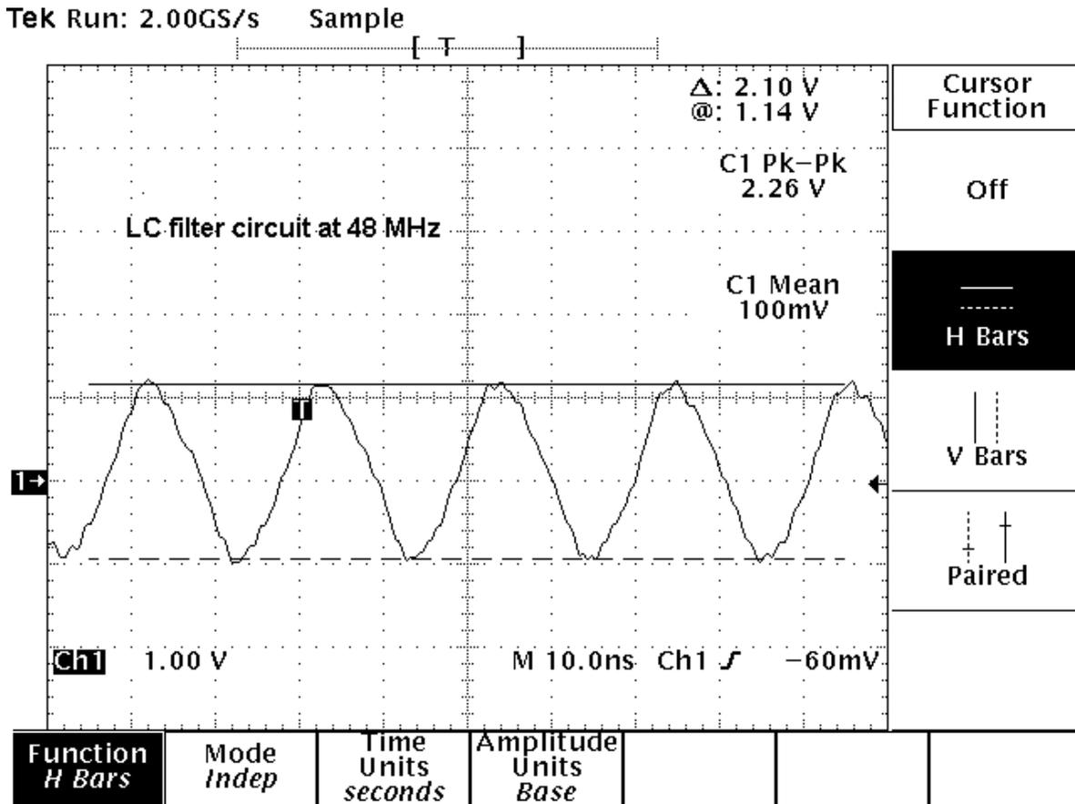
As seen here it has a mean of close to 0V (100mV shown) and a Peak to Peak voltage of around 2.3 volts. This is because it is capacitively coupled to pin 28 via the 10nF cap.
