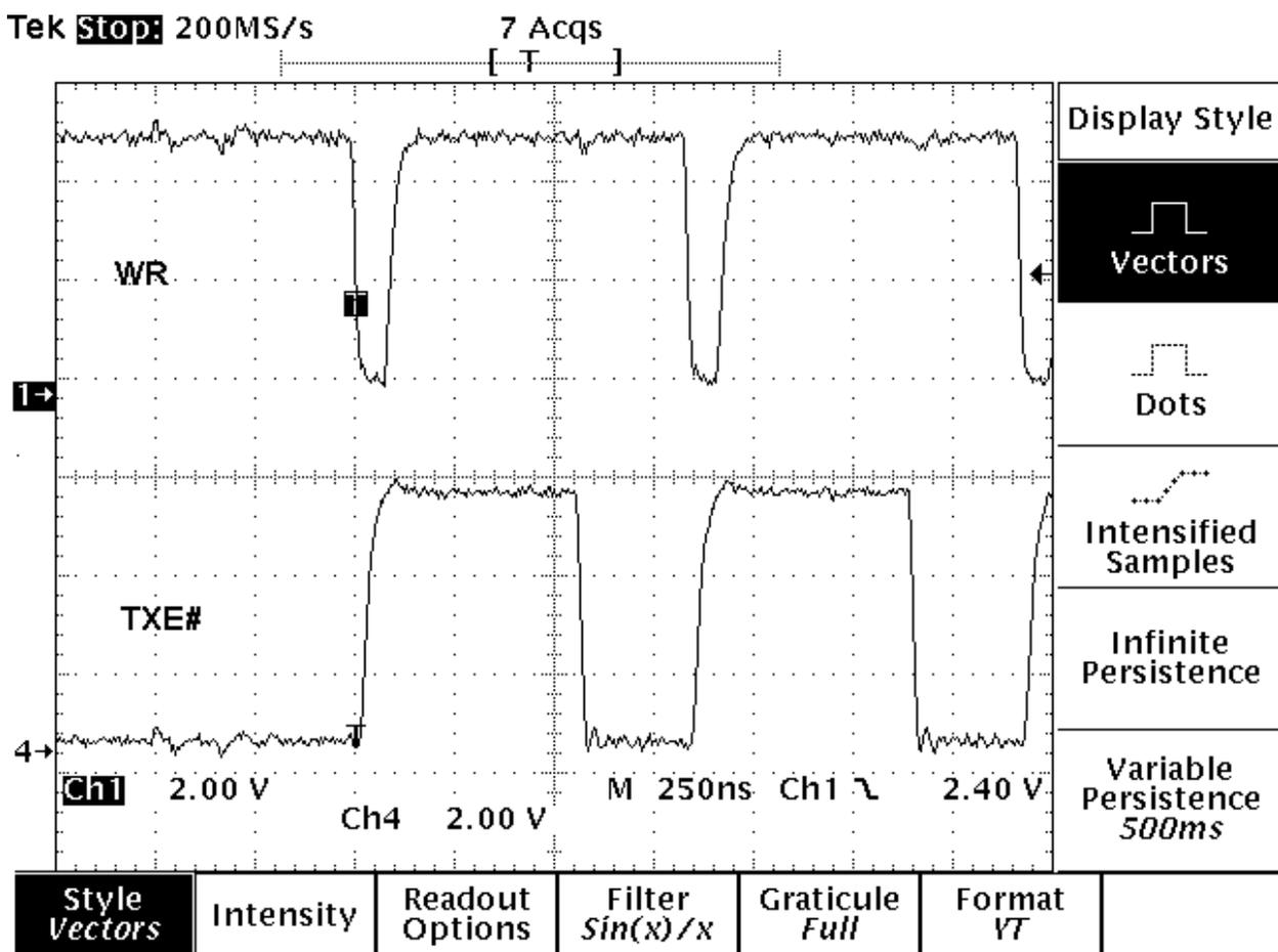
As can be clearly seen from the following trace, the TXE# signal becomes inactive ( high ) on the falling edge of WR. This example is using a single 12 MHz clock period for the WR inactive period, which gives a a negative pulse of approx. 80 nS.
