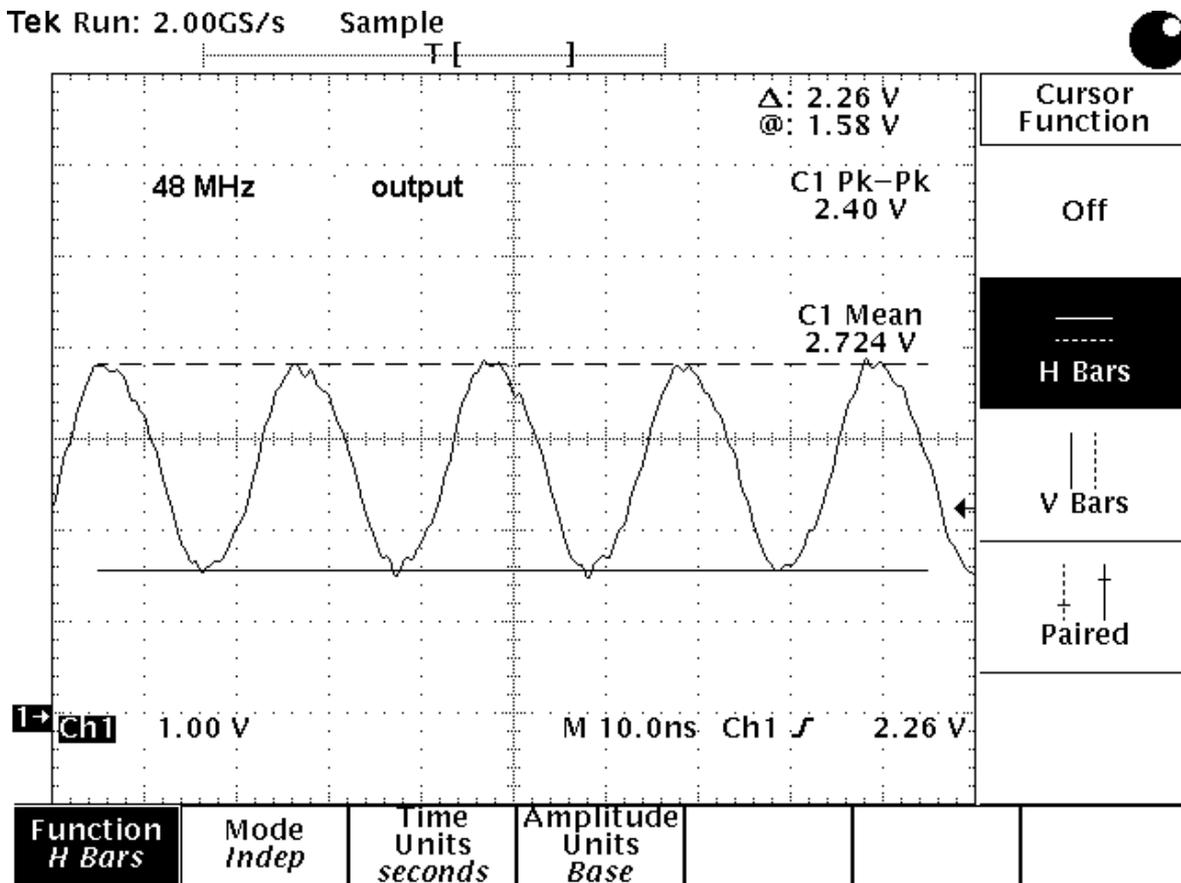
As seen here it has a mean of around 2.7 volts and a Peak to Peak voltage of around 2.4 volts.
